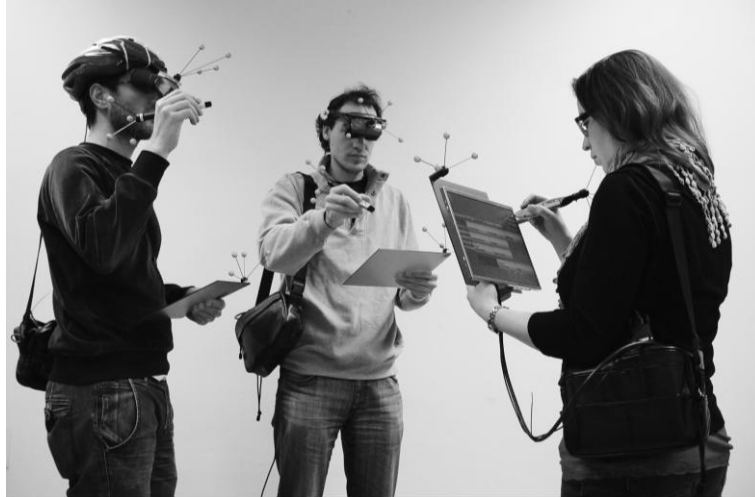
Figure 9. A wireless TFT display serves as a window into the virtual world for the teacher. Two wireless HMDs are used by students.
