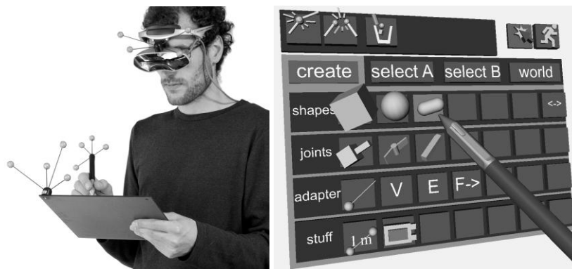
Figure 8. Left: Each user is equipped with input devices pen, PIP and head mounted display. Right: Example menu on the PIP.
